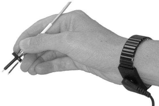
Figure 1. Correct method of holding the probe
