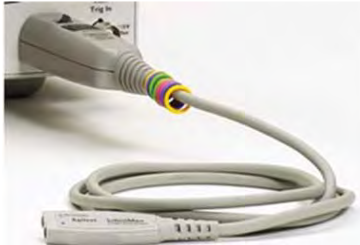
Figure 4. Many modern active probes rely on intelligent probe interfaces that provide power and serve as communication links between compatible probes and the scope.
