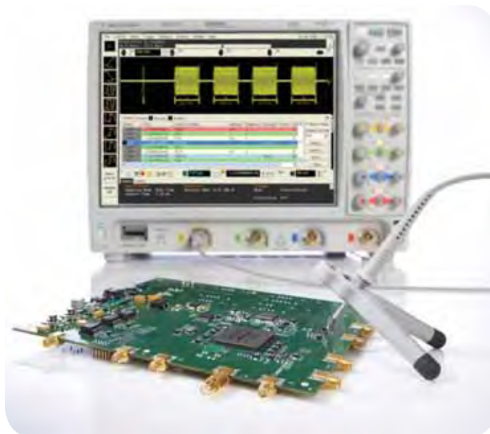
Figure 1. The passive voltage probe is the most commonly used type of scope probe today
