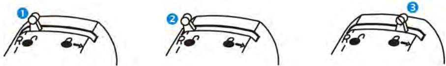
Figure 11 Properly Connecting a Probe to the Oscilloscope
