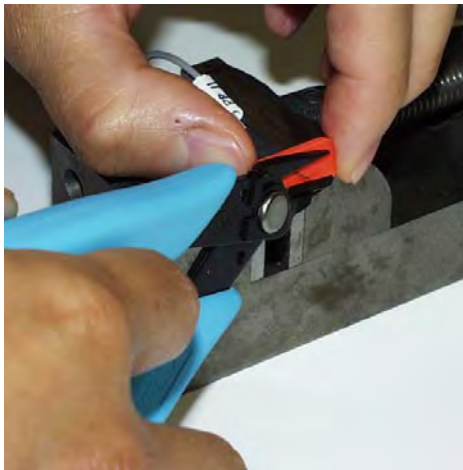
Figure 73 Cutting Wires Flush with Gauge
