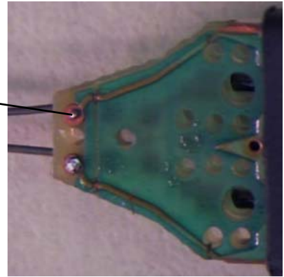
Figure 71 Wire Cut Flush with Solder pad
