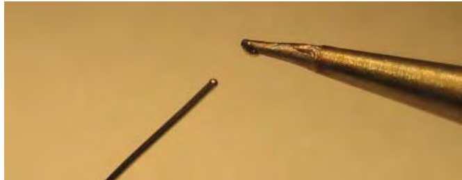
Figure 46 Small Amount of Solder Added to Soldering Iron Tip
