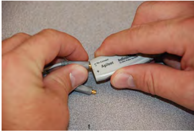
Figure 9 Improperly Disconnecting a Probe Head From an Amplifier
