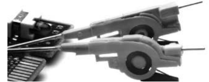
Extremely small-sized clips for probing PQFP and SOIC SMT packages
