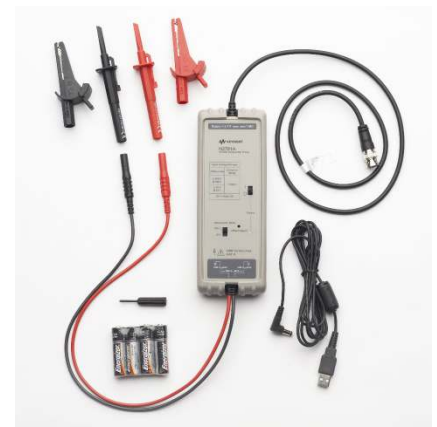
N2791A 25 MHz high voltage differential probe
