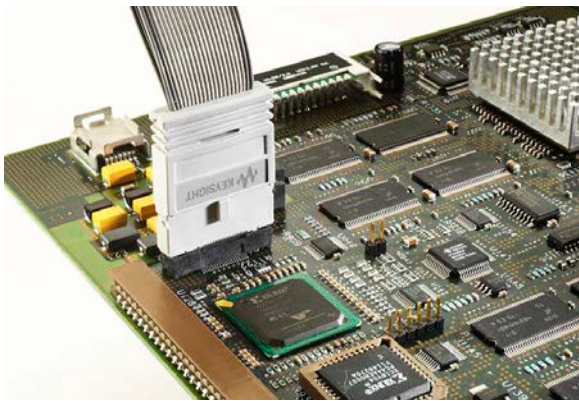
E5346A 34-channel Mictor connector probe
