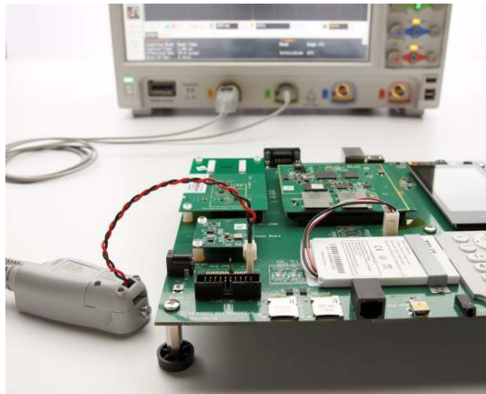
N2820A high-sensitivity 2-channel current probe
