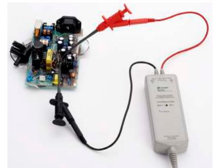
N2790A measuring a power supply signal
