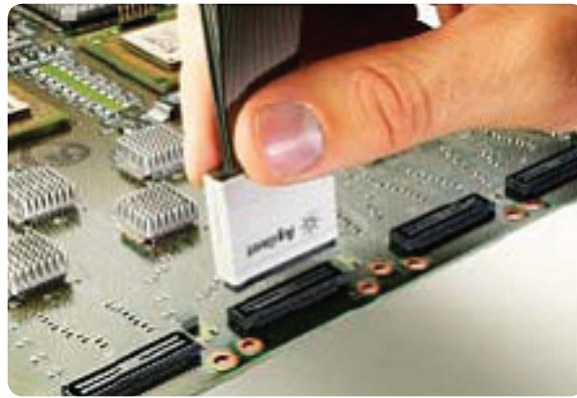
E5385A 34-channel Samtec connector probe
