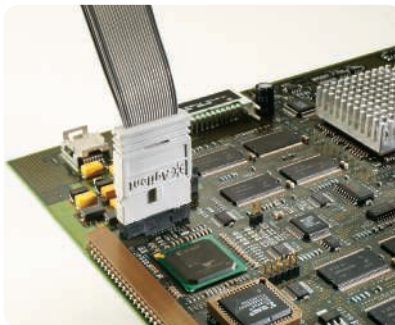
E5346A 34-channel Mictor connector probe
