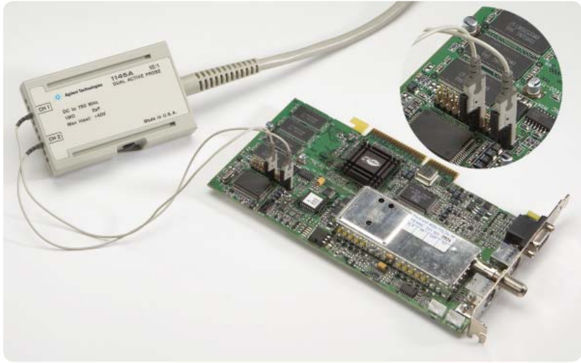
SMT grabbers provide solid connection to leads with down to 50-mil spacings
