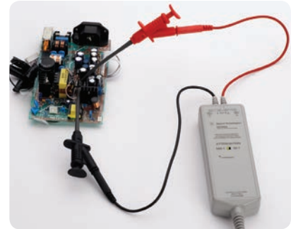
N2790A measuring a power supply signal
