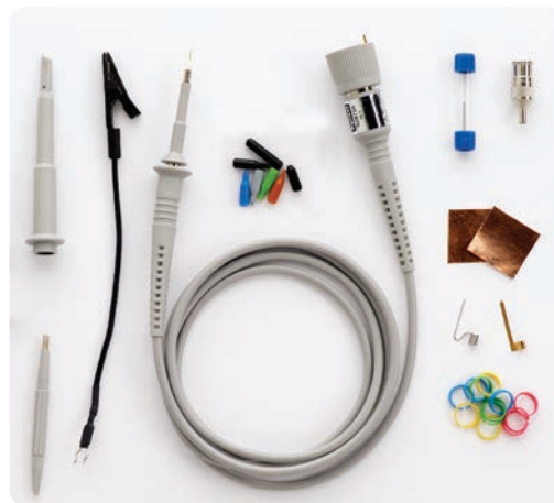
N2873A 500 MHz passive probe with standard accessories
