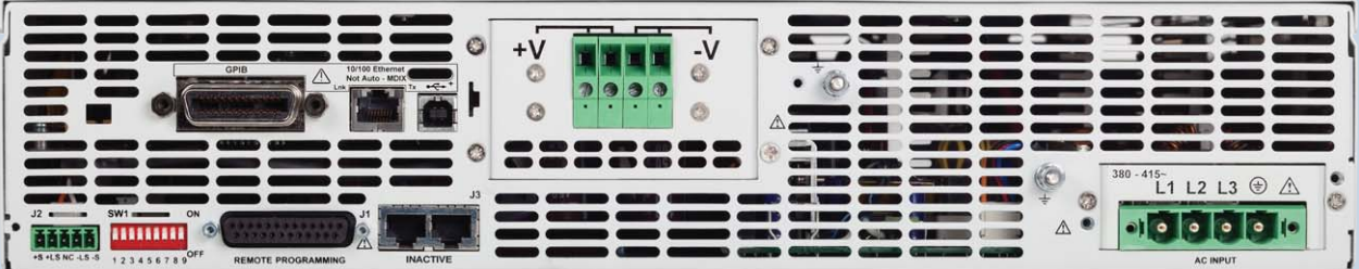
Rear panel with wire clamp connectors
