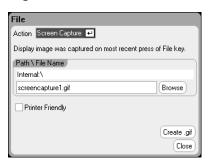
A copy of the current screen is saved whenever the File key is pressed.
