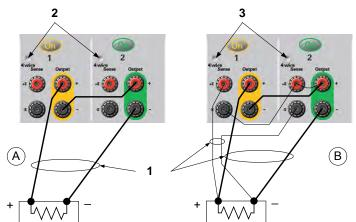
To program outputs connected in series, first program the current limit of each output to the total desired current limit point. Then program the voltage of each output so that the sum of both voltages equals the total desired operating voltage. The simplest way to accomplish this is to program each output to one half of the total desired operating voltage.
