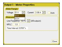
Meter Ranges - In the Voltage or Current dropdown menu, select the desired lower measurement range. Check the Auto box to enable measurement autoranging. The instrument automatically selects the best measurement range for the amplitude of the measurement.
