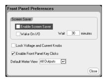
Check Enable Screen Saver to enable the screen saver. Uncheck to disable the screen saver. When enabled, enter a value in minutes in the **Wait** field to specify the time when the screen saver will activate. The wait can be set from 30 to 999 minutes in 1 minute increments.
