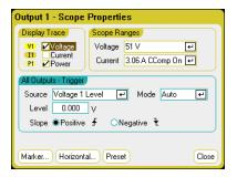
In the **Display Trace** area, select which traces to display for the output. If no box is checked, no traces will be displayed for that output. Voltage, current, and power traces can be displayed simultaneously only on Agilent Models N676xA and N678xA SMU, as these models have simultaneous voltage and current measurement capability (see chapter 1, "Power Module Features"). All other power modules can display either voltage or current traces, but not simultaneously.
