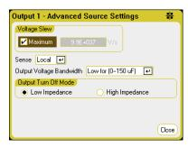
**Voltage Slew** - The voltage slew rate determines the rate at which the voltage changes to a new setting. To program a voltage slew rate, enter the rate (V/s) in the **Voltage Slew** field. Check **Maximum** to program the fastest rate. For Agilent Models N678xA SMU, the voltage slew control is only avilable in Voltage priority mode.
