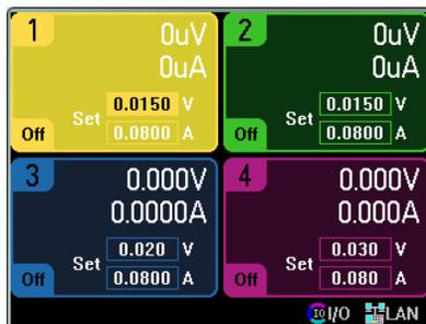
Press one of the four **On** keys to enable an individual output. In Meter View the DC Power Analyzer continuously measures and displays the output voltage and current of each output.
