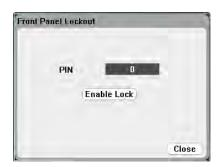
In the **PIN** text box, enter the numeric password that you wish to use to *unlock* the front panel. Then click **Enable Lock** to lock the front panel keys. A dialog prompting the user to unlock the front panel appears every time a key is pressed. Enter the password to unlock the front panel.
