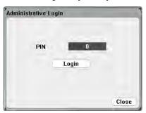
As shipped from the factory, the password is 0 (zero). If the PIN field shows 0; simply select the **Login** button and press [Enter].
