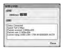
To change the GPIB address, use the numeric keys to enter a value in the GPIB address field. Valid addresses are from 0 to 30. Press Enter to enter the value.
