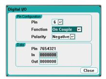
Select pin 6 from the **Pin** dropdown list. Then select the On Couple function for the pin the from the **Function** dropdown list.
