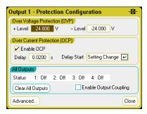
Over Voltage Protection - Over-voltage protection disables the output if the output voltage reaches the OVP level. To set the overvoltage protection, enter an over-voltage value in the **+Level** field.
