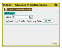
**All Outputs** – for all outputs you can program the **Inhibit** input (digital pin 3) on the rear panel to act as an external protection shutdown signal. The behavior of this signal can be set to either Latched or Live (non-latched). Off disables the remote inhibit. Refer to Appendix C for further information.
