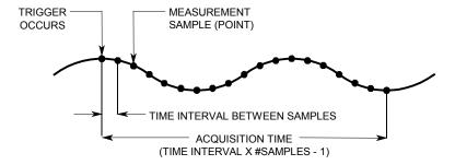
You can vary the measurement data sampling rate using the following commands. For example, to set the time interval to 60 microseconds with 4096 samples, use:
