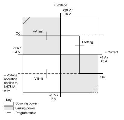
The heavy solid line illustrates the locus of possible operating points as a function of the output load. As shown by the vertical portion of the line, the output current remains regulated at its programmed setting as long as the output voltage remains within the positive or negative voltage limit setting. A CC (constant current) status flag indicates when the output voltage is within the limit settings.
