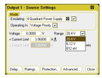
Voltage or Current Range - For outputs with multiple ranges, you can select a lower range if you need better output resolution. Use the navigation keys to highlight either the voltage or current **Range** field. Press the Enter key to access the dropdown range list. Use the navigation keys to select the desired output range.
