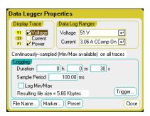
In the **Display Trace** area, select which traces to display for the output. If no box is checked, no data logging will occur on the output.
