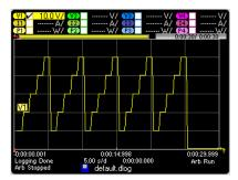
A message will indicate that the logged data has been saved in a file named default.dlog. If you wish to save the data under a different filename, you must specify the filename before the data logger runs. Select the Filename button located in the Datalogger Properties dialog to specify a filename.
