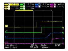
Note that the delay for output 1 does not start until 57 milliseconds have elapsed. This is because the internal delay for the mainframe used in this example is 57 milliseconds. This built in delay precedes any user-defined delays that have been programmed.
