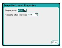
The **Sample Points** field lets you specify the number of points in a scope trace. The maximum number of points that can be specified depends on the number of scope traces that have been enabled. The minimum number of points that can be specified is 1024.
