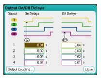
All power modules have an internal turn-on delay that applies from the time that the command to turn on the output is received until the output actually turns on. This turn-on delay is automatically added to the **On Delays** values. The turn-on delay does not apply when outputs turn off. To view the delay, select the Output Coupling button.
