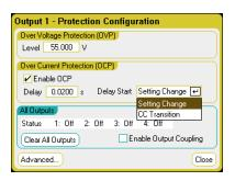
You can specify if the delay timer is started by *any* transition of the output into CC mode (select **CC Transition**), or if the delay timer is started at the end of a *settings* change in voltage, current, or output state (select **Settings Change**).
