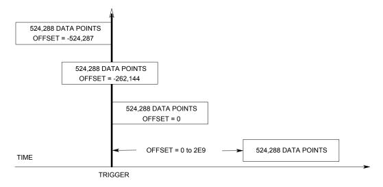
The following command offsets the beginning of the acquisition buffer relative to the trigger by 100 points on channel 1:
