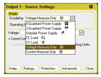
The **Voltage Measure Only** selection emulates a voltmeter. Current priority mode is set by default. The +/- Voltage Limits are set to their maximum values. No additional settings are required.
