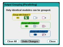
Grouped outputs are controlled using the output number of the **lowest** output in the group. As shown in the following figure, output 1 is grouped with output 2 and output 3 is grouped with output 4.
