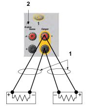
This minimizes mutual coupling effects and takes full advantage of the DC Power Analyzer's low output impedance. Keep each pair of wires as short as possible and twist or bundle them to reduce lead inductance and noise pickup. Keep the load leads under 14.7 meters (50 feet) per lead because of inductance effects.
