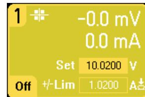
Lastly, you can press the **Settings** key to access the Source Settings window. Use the navigation keys to highlight the **Voltage** or **Current** fields. Then enter the voltage and current values with the numeric keys. You can use the Voltage and Current knobs to adjust the values in the Voltage and Current fields. Press **Enter** to enter the value.
