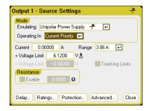
Resistance - This is only available on Agilent Model N6781A. Output resistance programming is primarily used in battery emulation applications, and only applies in Voltage Priority mode. Values are programmed in Ohms, from  $-40 \text{ m}\Omega$  to  $+1 \Omega$ .
