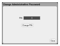
If the password is lost or forgotten, access to the Administrative Tools menu can be restored by setting an internal switch to reset the password to 0. If the message "Locked out by internal switch setting" or "Calibration is inhibited by switch setting" appears, the internal switch is set to prevent the password from being changed (Refer to the Service Guide).
