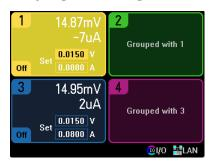
To return grouped outputs back to an ungrouped state, turn the output off and remove the parallel connections between the outputs. Then uncheck the check boxes. Then cycle AC power to the unit for the grouping or ungrouping changes to take effect. Grouped settings are saved in non-volatile memory.
