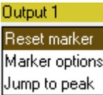
Push the <code>Enter</code> key to Reset the marker. Push <code>Enter</code> again to undo the reset action. Scroll down and select Marker options to access the Scope Marker Properties window. Scroll down and select Jump to peak to move the marker to the peak measurement point of the trace. |
