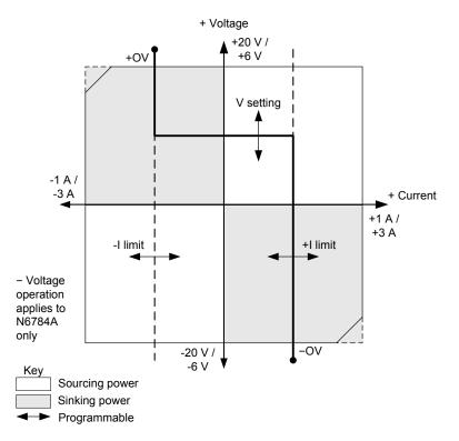
The heavy solid line illustrates the locus of possible operating points as a function of the output load. As shown by the horizontal portion of the line, the output voltage remains regulated at its programmed setting as long as the load current remains within the positive or negative current limit setting. A CV (constant voltage) status flag indicates that the output current is within the limit settings.
