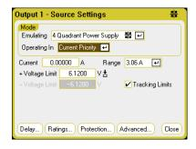
Operating in - selects either Voltage Priority or Current Priority. In voltage priority the output is controlled by a bi-polar constant voltage feedback loop, which maintains the output voltage at its positive or negative setting. In current priority the output is controlled by a bipolar constant current feedback loop, which maintains the output source or sink current at its programmed setting.
