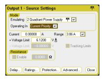
Operating in – selects either Voltage Priority or Current Priority. The other settings in 2-quadrant mode are the same as the settings in 4-quadrant mode except that you cannot program negative voltages or negative voltage limits. Because of this, voltage tracking is not available in Current Priority mode. Note that the negative voltage limit is fixed at -10 mV.
