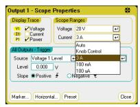
Selecting **Knob Control** allows the **Vertical Volts/Div** knob on the front panel to automatically select lower measurement ranges at lower measurement resolutions. For higher measurement resolution a higher range is automatically selected. The present range is displayed on the lower left corner of the Scope View window.
