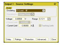
In CC load mode you can specify the input Current and Range as well as the + Voltage Limit. Current Priority mode is locked. Remember to set the input current to a negative value. The + Voltage Limit should normally be set to its maximum value. The – Voltage limit is not programmable. In Meter mode, the measurement polarities and current settings are shown as negative values.
