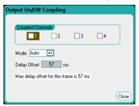
Normally, the firmware automatically calculates the delay offset based on the longest minimum turn-on delay of the installed power modules. However, if you will be excluding some outputs from participating in an output on/off delay sequence as described Step 3, the delay offset may be different based on the outputs that you will actually be sequencing. The minimum turn-on delays of the power modules are documented in the Agilent N6700 Modular Power System Family Specifications Guide.
