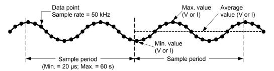
The fastest sample period that can be programmed for continuouslysampled measurements is 20.48 microseconds. However, this speed is only possible if *one* parameter is being measured. Note that you can measure up to 24 parameters (average voltage+min+max X 4 outputs, and average current+min+max X 4 outputs) with a corresponding decrease in measurement sample rate. The following typical sample periods are based on the number of parameters selected:
