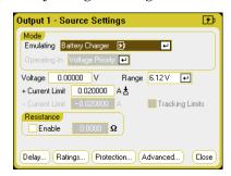
In Battery Emulator mode you can specify the battery voltage and range as well as the + and - current limits. The output resistance is programmable, from – 40 m $\Omega$  to + 1  $\Omega$ . Voltage Priority mode is locked. The voltage setting is limited to positive values. The + and current limits are set to their maximum values. The - current limit setting sets the current limit when the battery is being charged.
