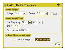
The instrument will continuously display the auxiliary voltage measurement on the front panel Meter View:
