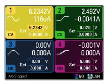
A single-output view displays more information about the selected output. Press the Meter View key to toggle between the two views.
