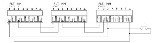
As shown in the figure above, you can also connect the Inhibit input to a manual switch or external control signal that will short the Inhibit pin to common whenever it is necessary to disable all output channels in the mainframe. Negative polarity must be programmed for all pins in this case. You can also use the Fault output to drive an external relay circuit or signal other devices whenever a user-definable fault occurs.
