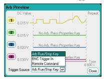
Arb Run/Stop key selects the front panel Arb Run/Stop key as the trigger source. This means that the Arb will be triggered as soon as you run it. BNC Trigger In selects the rear trigger input BNC connector as the trigger source. Remote command selects a remote interface command as the trigger source.
