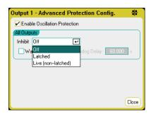
Select the **Inhibit** dropdown list. The inhibit signal can be live, latched, or off. The Inhibit mode is stored in non-volatile memory.
