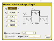
Use the **Advanced** button to specify what happens when the Arb sequence completes – select whether the output Returns to the DC Value that was in effect before the waveform started, or whether the output should remain at the Last Arb Value. Also specify if the Arb sequence should repeat, either continuously or only for a specified repeat count. A repeat count of 2 runs the Arb sequence twice.
