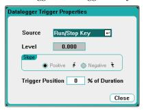
The **Source** dropdown list lets you select a trigger source. The same trigger source will be used to trigger all of the outputs that have been configured for data logging. Depending upon the selected trigger source, you can trigger the Data Logger as follows:
