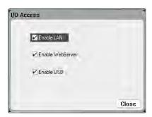
Check the Enable LAN box to enable the LAN. Uncheck this box to disable the LAN.
