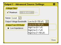
Select a bandwidth according to the following load capacitances and load lead lengths:
