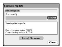
Click the Browse button and navigate to the firmware file on the External USB memory Device. Press the **Install Firmware** button to update the firmware.
