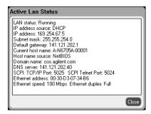
Note that the currently active LAN settings for the IP Address, Subnet Mask, and Default Gateway may be different from the settings specified in the "Modify LAN Settings" window - depending on the configuration of the network. If the settings are different, it is because the network has automatically assigned its own settings.
