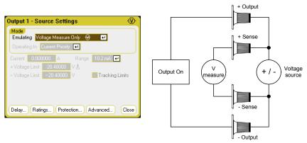
The Voltage Measure Only mode works best when the sense terminals are connected to the output terminals, either by connecting the sense and load leads to directly to the DUT, or by using the local sensing on the front panel. Note that the input impedance in Voltage Measure Only mode will be somewhere around 2000 pF depending on the grounding of the DUT. This may draw up to a few microamperes of current from the nodes that are being measured.
