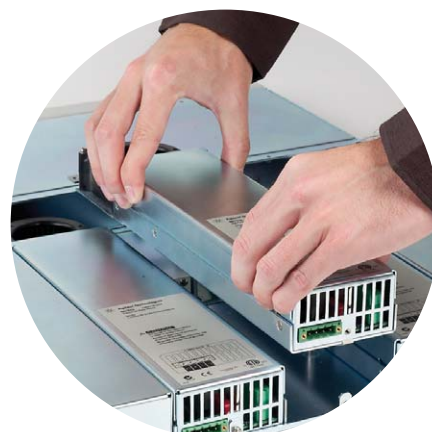
Figure 6c. User re-configurable modular system
