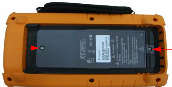
Figure 8-3 Remove battery cover screw
