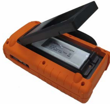
Figure 8-5 Remove battery pack cover without removing stand
