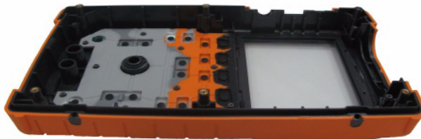
Figure 8-12 Remove keypad from the front cover
