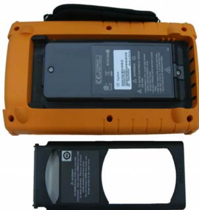
Figure 8-2 Disassemble the stand from the instrument
