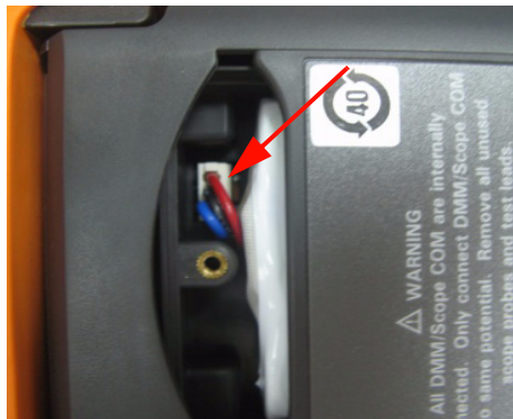
Figure 8-6 Unplug 2-wire connector with a tweezers.
