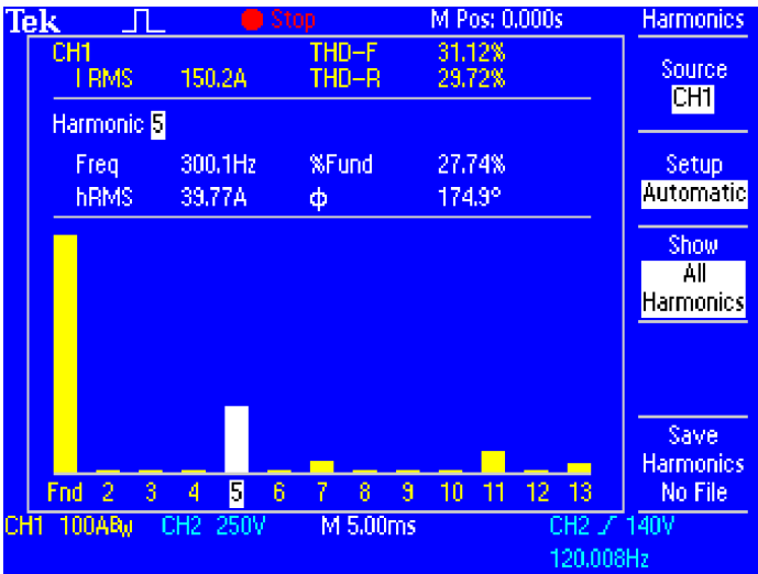
Conduct harmonic distortion measurements with TPS2PWR1 software.
