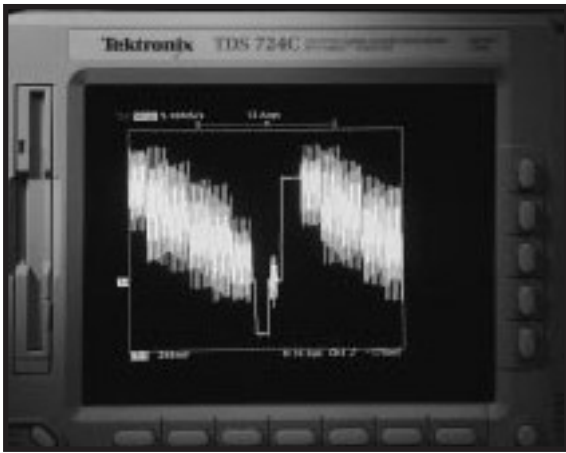
A traditional DSO is unable to display the details and dynamic changes of this composite video waveform.
