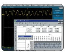
Open Windows Platform. TDS5000 Series waveform display with Excel window and ActiveX toolbar.
