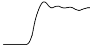
Long ground lead
