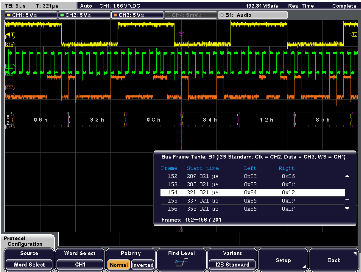
Fig. 11-22: Decoded I²S signal with frame table
