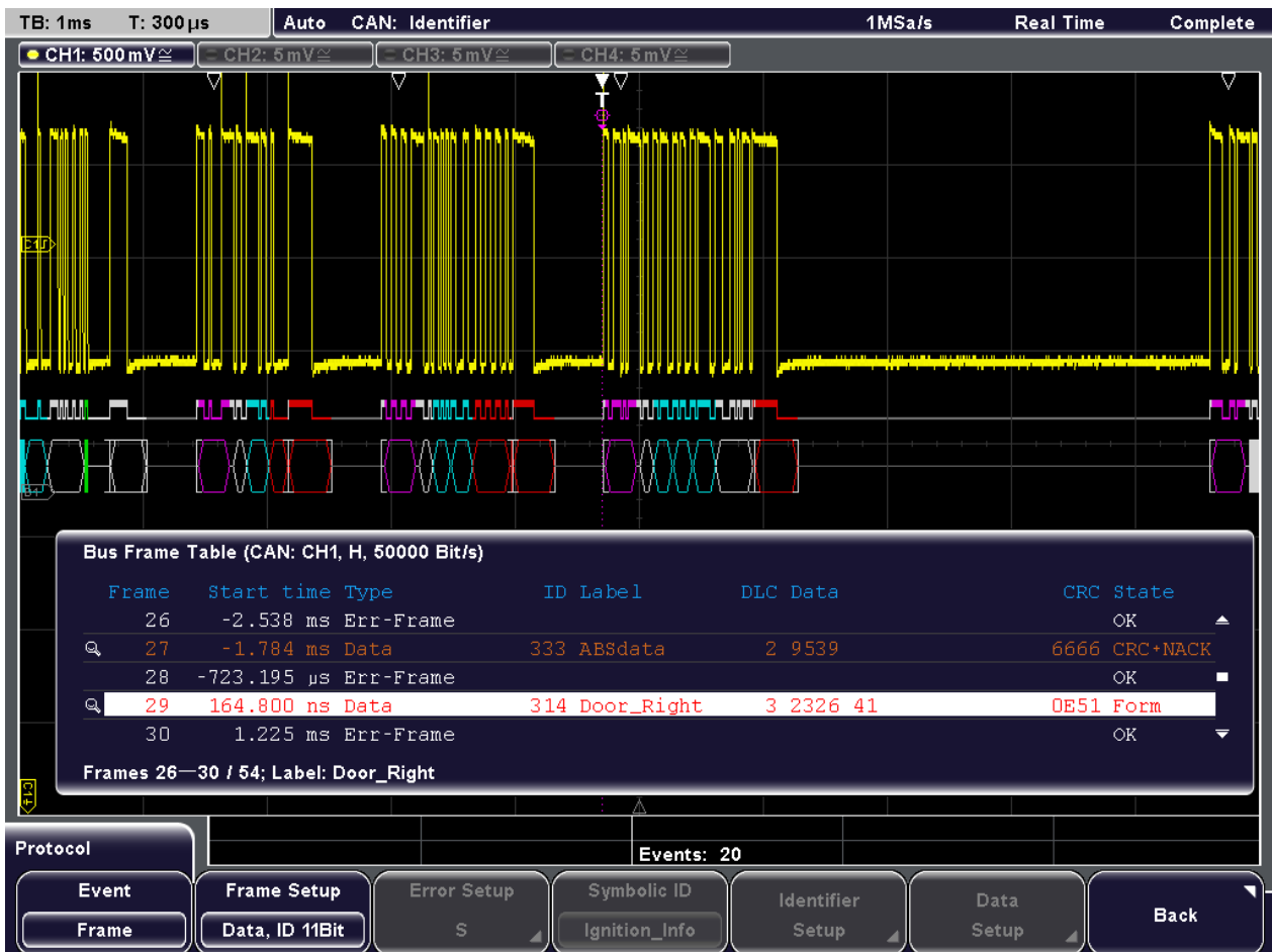
Fig. 11-13: Search for data frames with 11 bit identifier, search results are marked in frame table and on the decoded data
