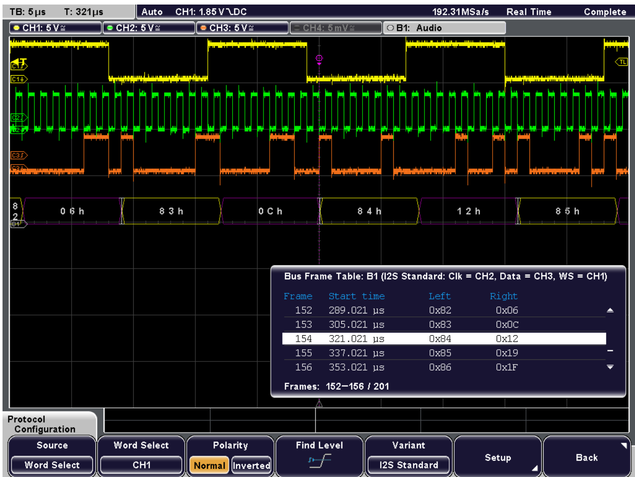
Fig. 11-22: Decoded I 2 S signal with frame table
