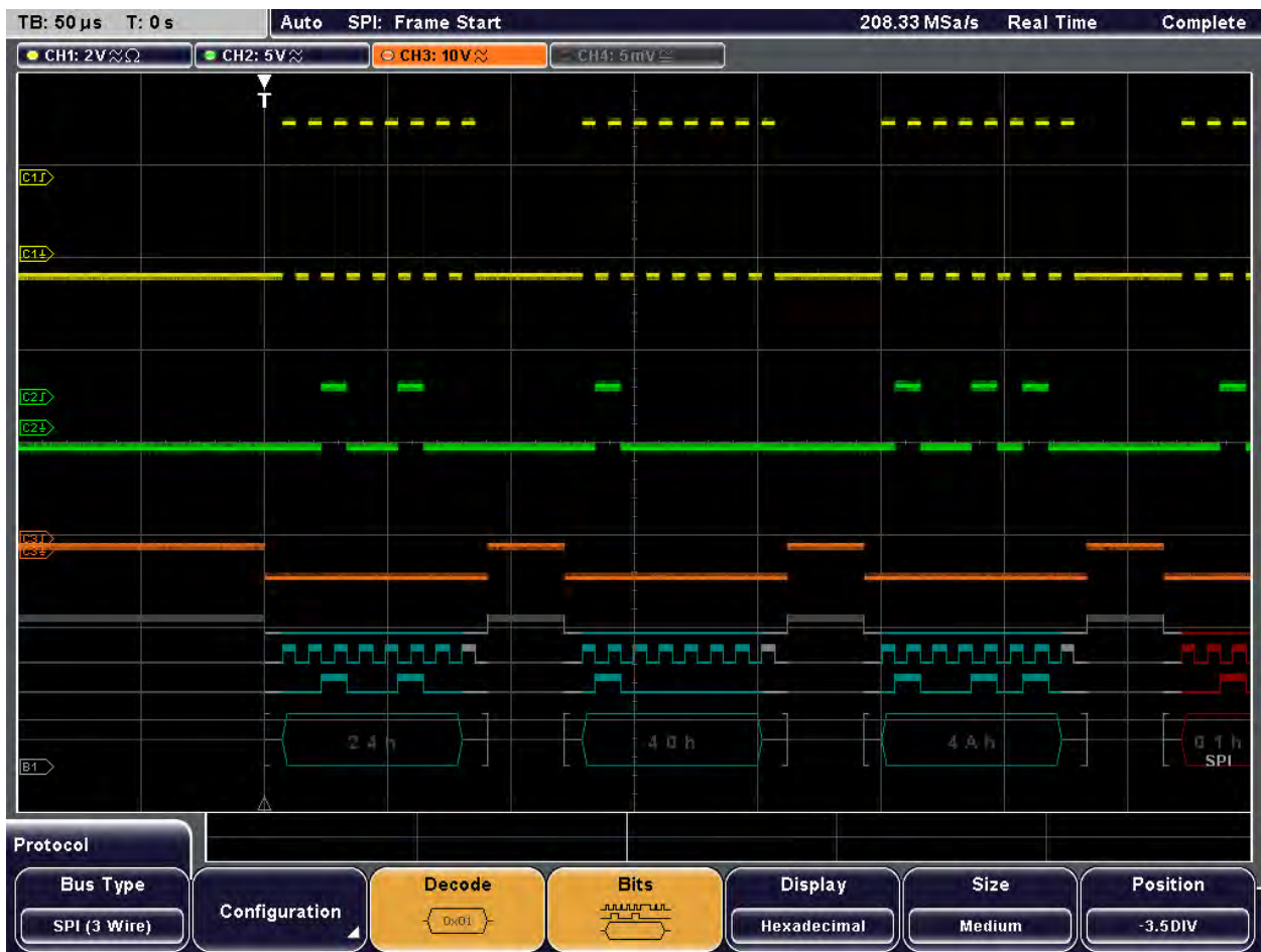
Fig. 11-2: Decoded SPI signal
