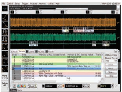
Trigger on and decode PCIe serial packets.
