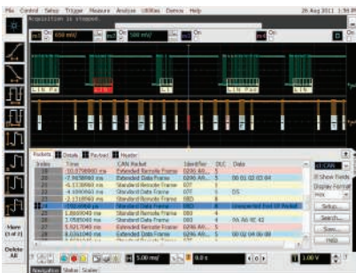
Trigger on and decode CAN, LIN and FlexRay serial packets.
