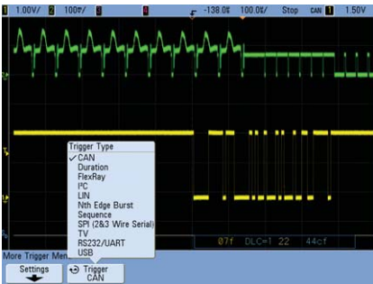
Trigger on and decode CAN serial packets.
