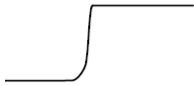
Signal with a short ground lead
