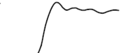
Signal with a long ground lead
