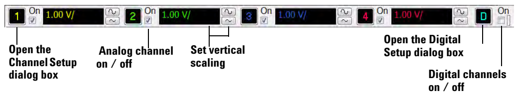
Figure 20 GUI Vertical Controls
