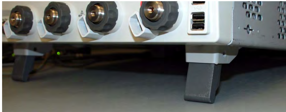
Figure 4 Flip-Out Tabs Under Front Feet
