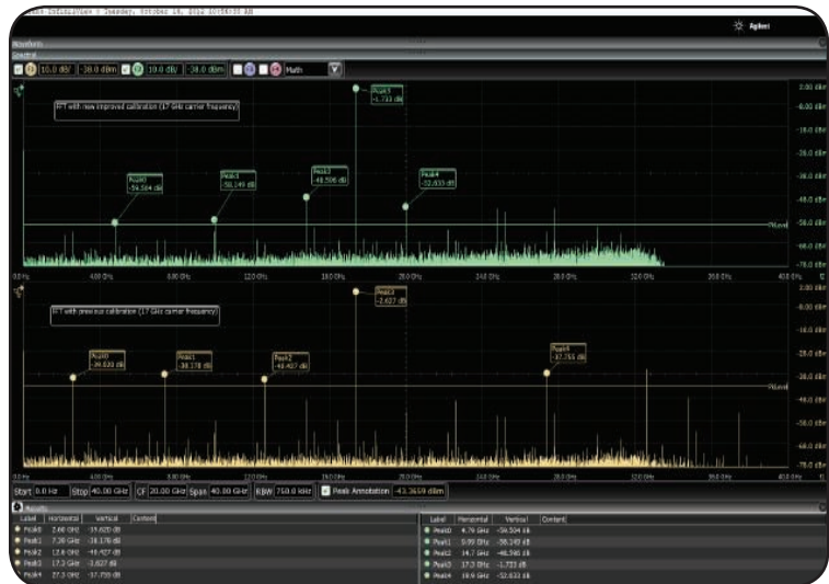
Improved calibration improves the spurious free dynamic range by up to 15 dBc
