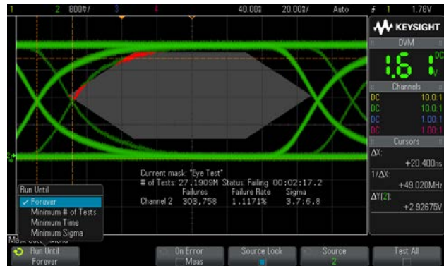
Mask test evaluated more than 27 million waveforms in just over two minutes.
