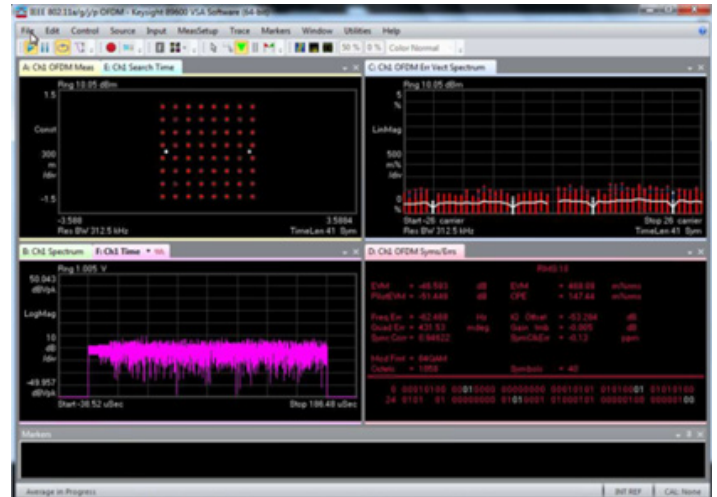
Using data acquired from S-Series, VSA shows an EVM for IEEE 802.11 QAM 64 of 0.47%.
