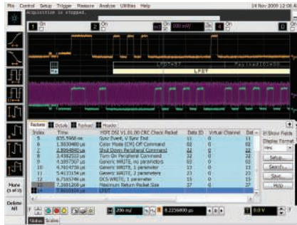
Trigger on and decode MIPI packets.
