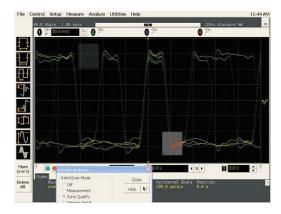
The "true" ease of use. Just draw boxes and the scope will trigger. The industry's only software event finder, InfiniiScan event identification tool provides the next level of ease of use for the scope triggering system.
