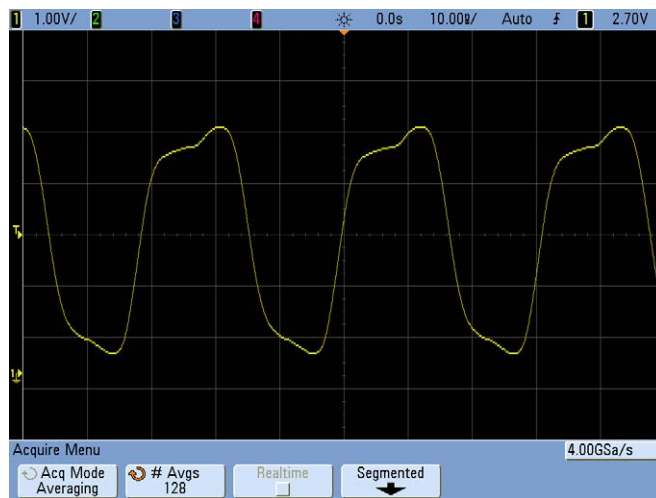
Figure 34 128 Averages used to reduce random noise
