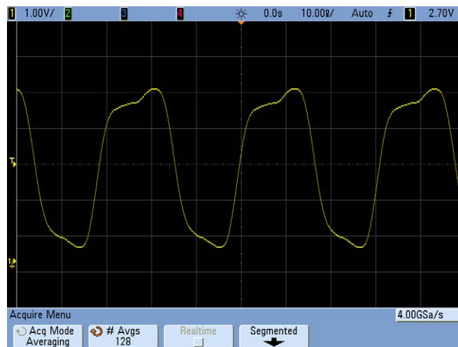
Figure 34 128 Averages used to reduce random noise
