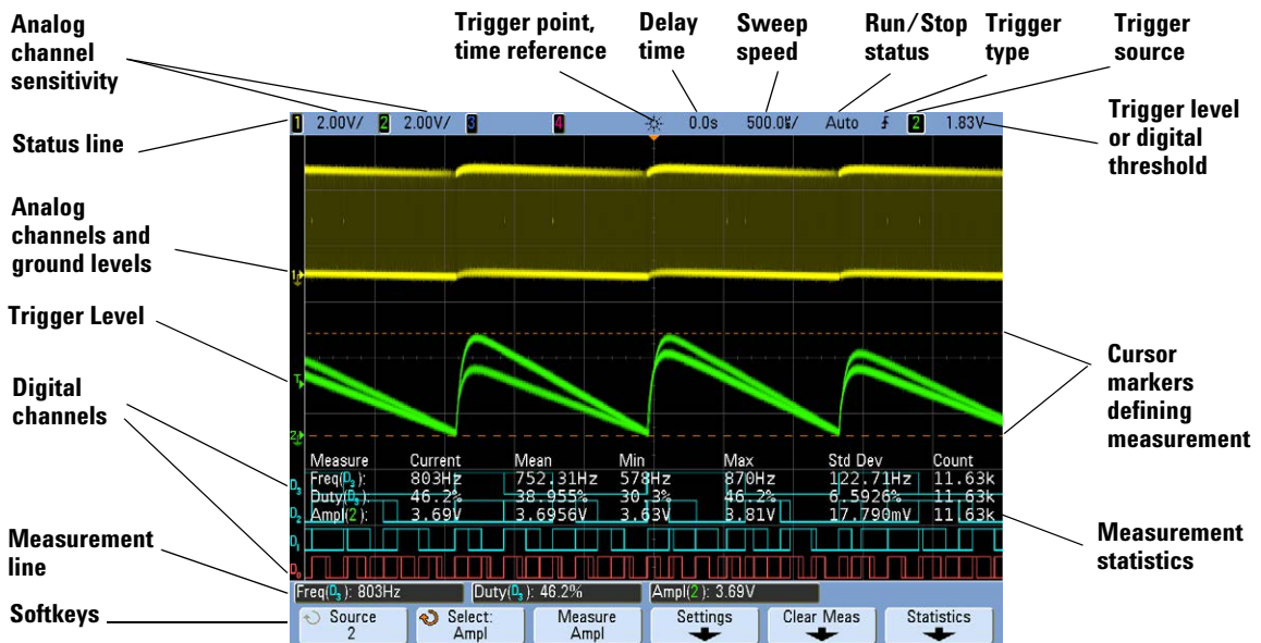
Figure 1 Interpreting the oscilloscope display
