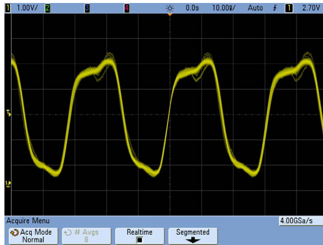
Figure 34 128 Averages used to reduce random noise
