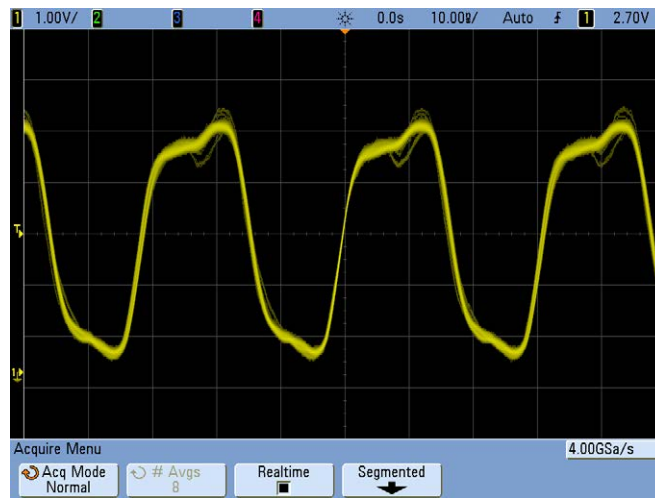
Figure 34 128 Averages used to reduce random noise
