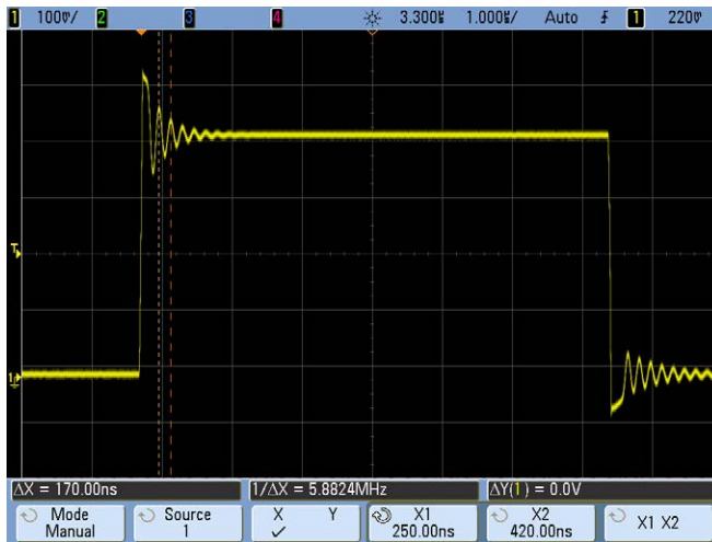
CURSORS MEASURE FREQUENCY OF PULSE RINGING
