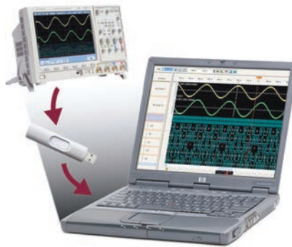
Figure 15. View and analyze previously acquired scope data on a PC-based offline tool
