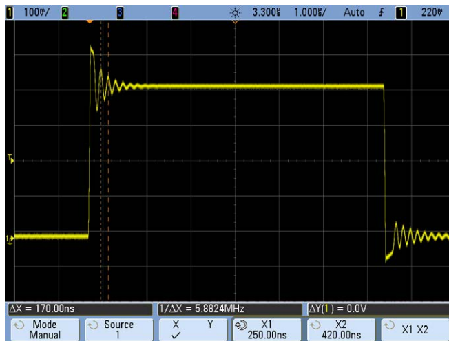
CURSORS MEASURE FREQUENCY OF PULSE RINGING
