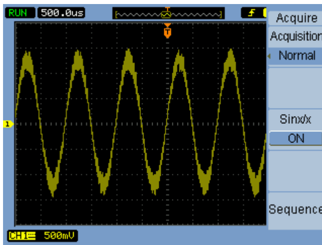
Figure 31 Noisy Waveform Without Averaging
