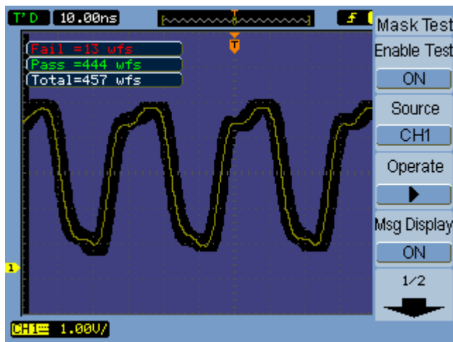
Figure 54 Mask Test Display
