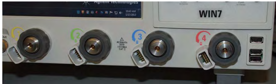
Figure 3 90000 X-Series Oscilloscope Probe Connectors
