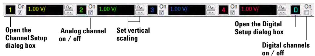
Figure 20 GUI Vertical Controls
