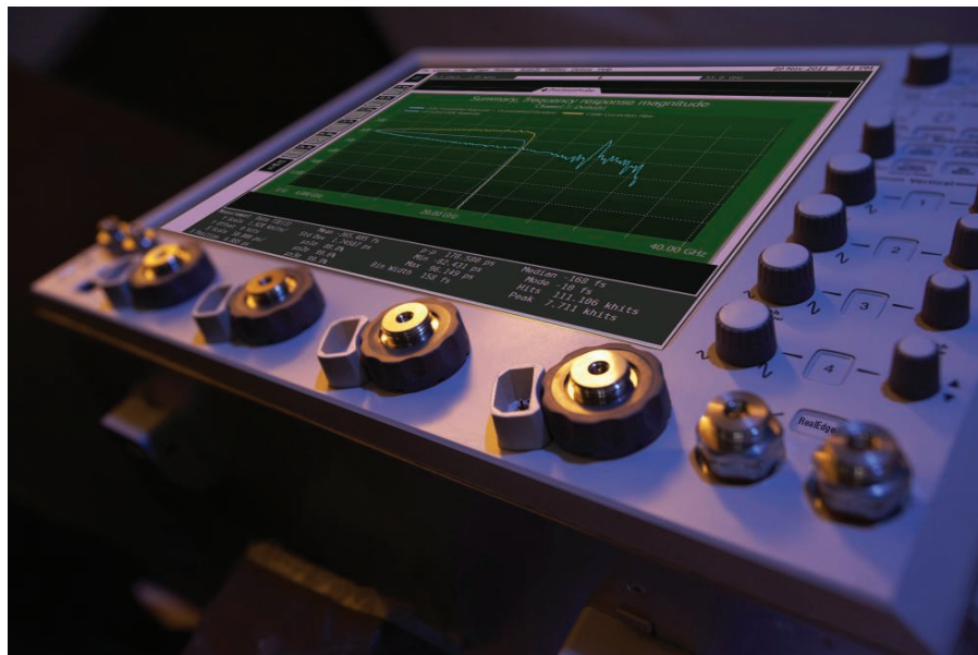
PrecisionProbe software characterizes cables to 63 GHz
