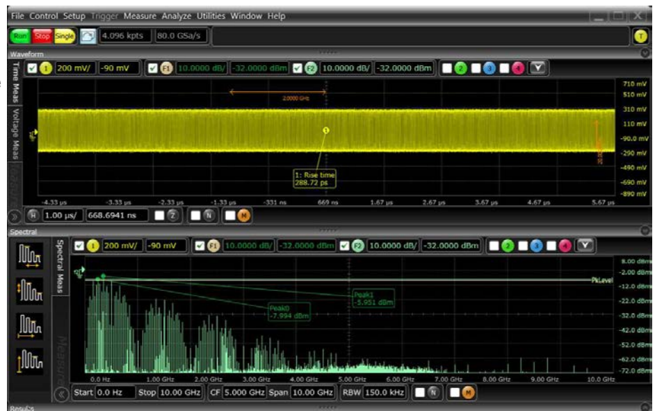
Agilent's InfiniView software provides full off line capability including FFTs
