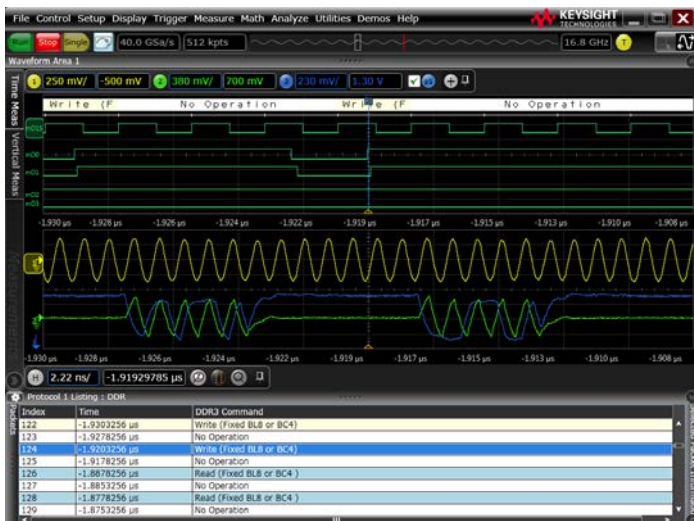
DDR3 protocol decode and write command trigger.
