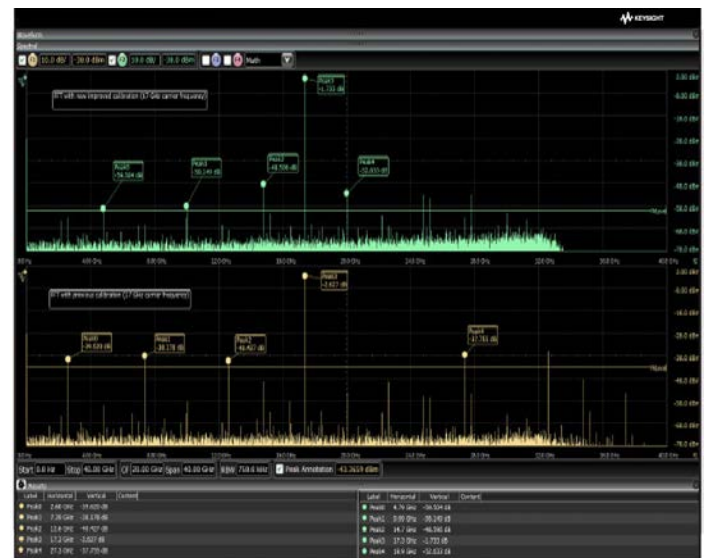
Improved calibration increases the spurious free dynamic range by up to 15 dBc.
