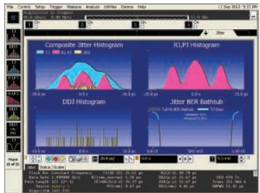
Analyze jitter plus RJ/DJ separation.
