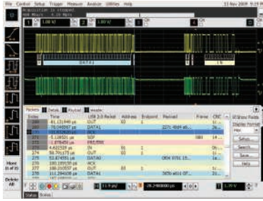
Trigger on and decode USB packets.
