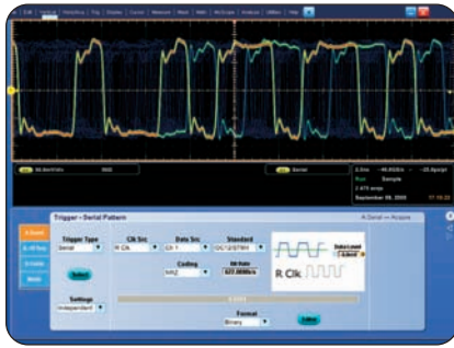
► Serial pattern triggering to debug pattern-dependent issues.
