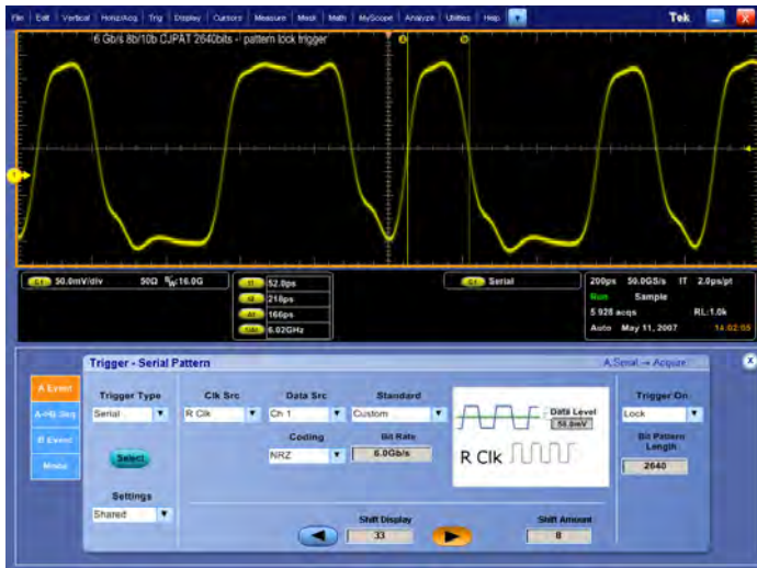
NRZ Pattern Lock Triggering of a 640-bit long serial test pattern SATA 6Gbps
