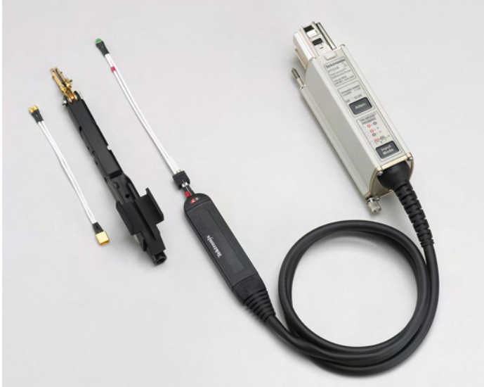
P7500 TriMode probes simplify complex measurement setups.
