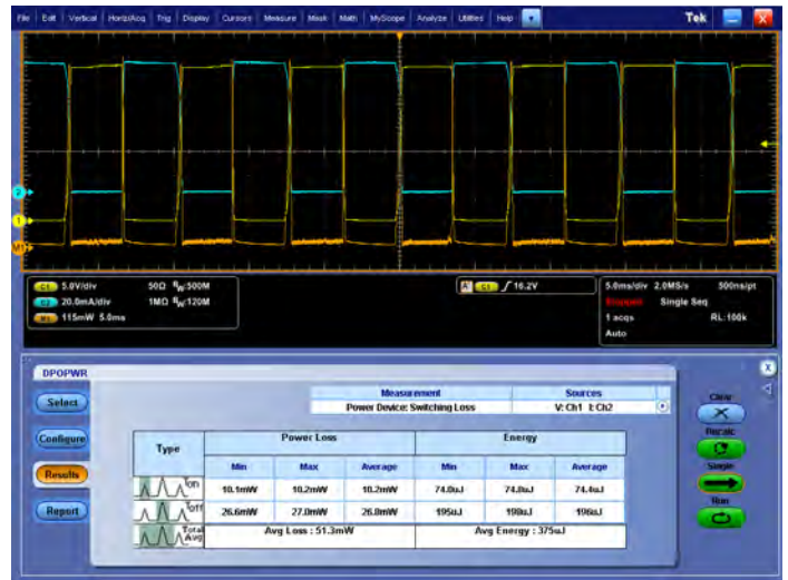
Switching Loss measurements. Automated power measurements enable quick and accurate analysis of common power parameters.
