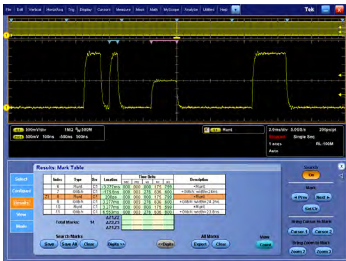
Search – Results of an advanced search for a runt pulse or a narrow glitch within a long waveform record. Each instance of the runt or glitch is automatically marked for easy reference.
