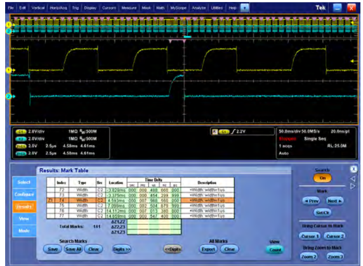
Search step 2: Advanced Search and Mark automatically searches through the record and marks each event with a solid colored triangle. You can then use the Previous and Next buttons to jump from one event to the next.
